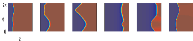
Fig.1 Typical non-rotating patterns superimposed on an axial oscillating front in a 2-D cylindrical shell model with oscillatory kinetics showing several temperature snapshots during one period.
